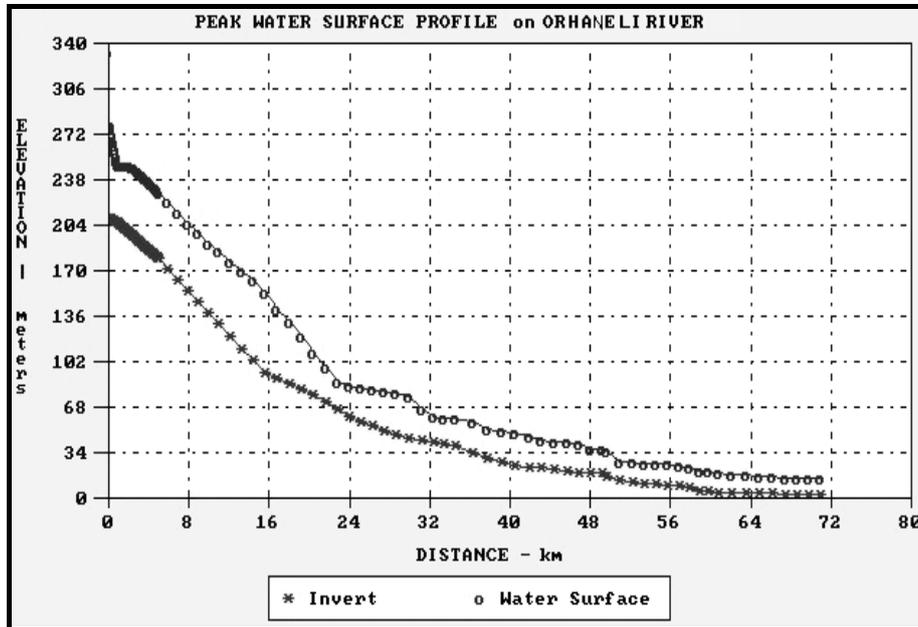
Figure 7. Peak Water Surface Profile on Orhaneli River
