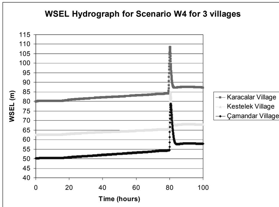
**Figure 8.** WSEL Hydrograph in Three Villages for Scenario W4
