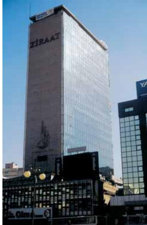
*Emek Office Building project, which has been obtained as a result of a competition and constructed by Retirement Fund, has become the symbol of Ankara of that time by coming near to the examples in the West with its prismatic form as relation of low and high blocks and two façades of which are reinforced concrete shear wall, and other two is aluminum-glass cladding system detached from the structure.*
