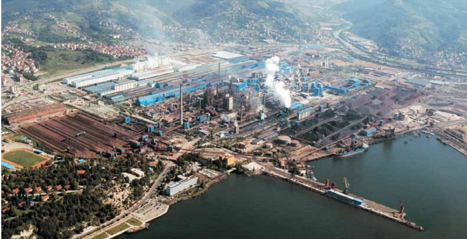
*The production capacity of Erdemir was 470,000 ton/year for raw steel, 110,000 ton/year for blum and 268,000 ton/year for steel sheet and in total for steel production 378,000 ton/year.*
