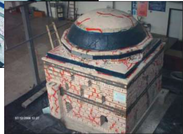
•Kaynak: Shaking table tests on the large scale model of Mustafa Pasha Mosque without and with FRP
