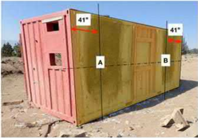
Location of Deflection Control Points on Front Wall of Ground Unit
