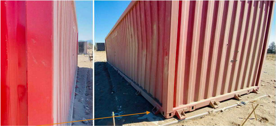
Anchored Unit - Deformation Along Front Face (left, right) and Undeformed Side Face (right)
