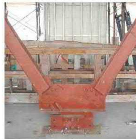
Friction damper in chevron bracing (inverted)
