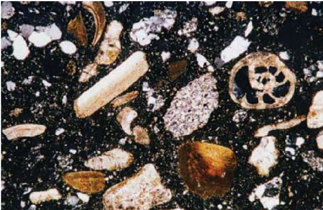
Petrographic image captured of the bridge concrete revealing seashells. Comparable shell material can be identified at the nearby Barleycove beach.
