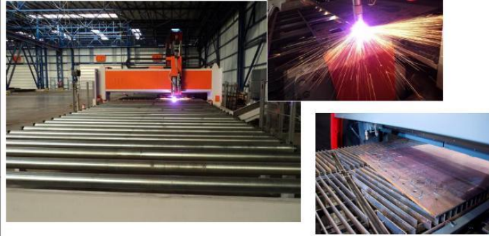
Steel Service and Process Centre Plate Processing: Drilling and Plazma/Oxy Cutting
