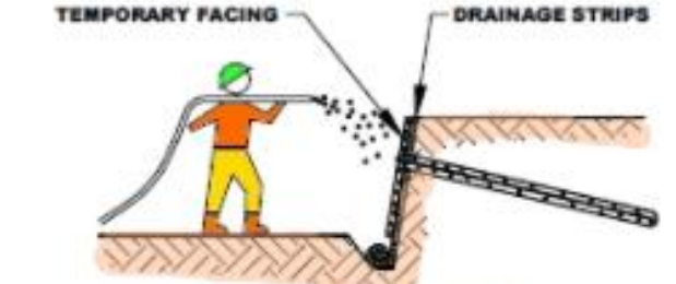
STEP 4. PLACE TEMPORARY FACING (INCLUDES SHOTCRETE, REINFORCEMENT, BEARING PLATE, HEX NUT, AND WASHERS INSTALLATION)
