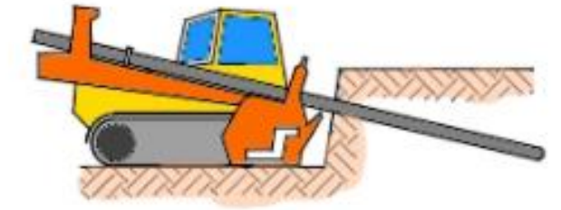
STEP 2. DRILL NAIL HOLE
