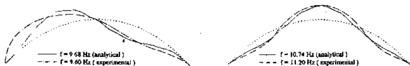
Fig 6 Mode shapes of the model determined analytically, i.e. experimentally
